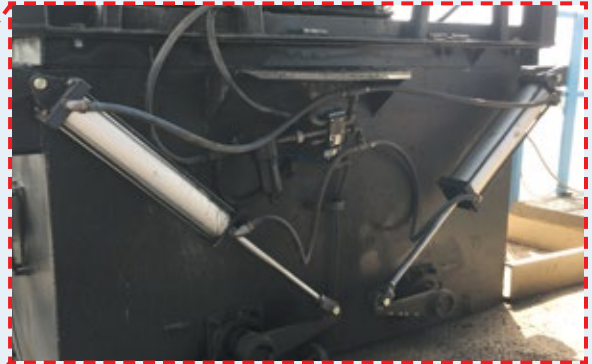
SHOWN: 4 x 16 batcher cylinders
